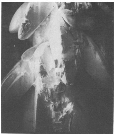
Figure 10 Enlarged SEM view of top of a dendrite, \times 150 .
