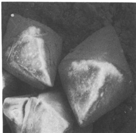
Figure 11 Octahedral bipyramid \text{BaMoO}_4 crystals nucleated in control tubes without electric field, \times 300 .
